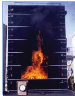
Full-scale Fire Test UBC 17-6 / UBC 26-4
