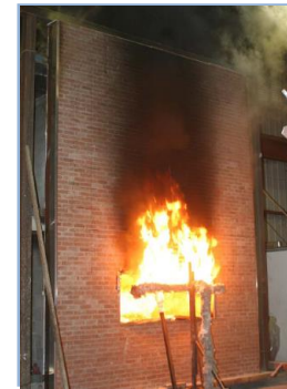
Reduced-scale Fire Test UBC 26-9 / NFPA 285
